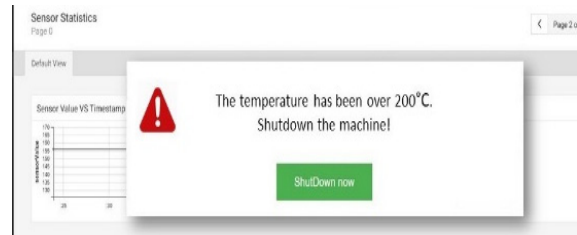
Figure 9: Notification alert for temperature value greater than 200°C and action confirmation.
